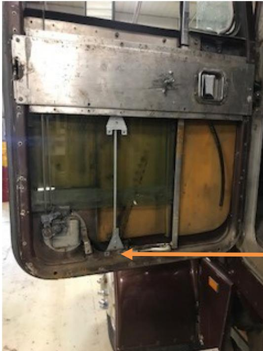
9. Test fit window channel to door and mark with sharpie
